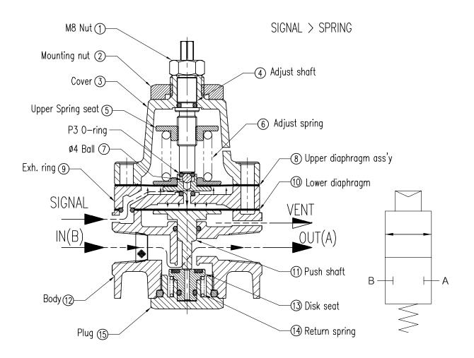
If the signal pressure is larger than the setting pressure (6 adjustment spring force), the signal pressure lifts the (8) upper diaphragm assembly upward. The signal pressure pushes the (1) push shaft and (3) disc seat down while pushing the (10) lower diaphragm through the middle hole. As a result, the IN (B) port is connected to the OUT (A) port.
